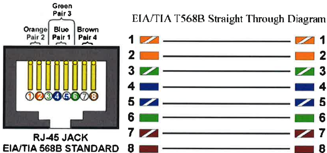
FIGURE 1: TELEPHONE LINES SHALL BE CONNECTED TO PAIR ONE (1) ON PINS 4 AND 5, IN THE CENTER OF THE RJ-45 JACK. EVERY PHONE LINE SHALL BE CONNECTED USING TIP, ON PIN FIVE (5) AND RING, ON PIN FOUR (4) IN THE RJ45 VOICE PATCH PANEL MOUNTED IN THE TOP OF THE 19” RACKS IN THE TELECOMMUNICATIONS ROOM(TR).
