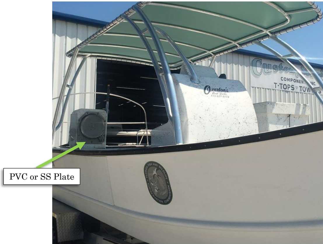
Figure 5. Example of Hauler mount, T top size and hull protection
