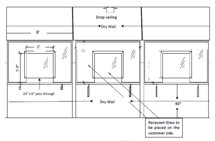
Lessor to provide counter at customer service window to include a 40" high, 24" wide and shall span continuous across all of the customer service windows. Of the 24" wide, 6" shall overhang into the employee area and the other 18" in the lobby/reception area.
