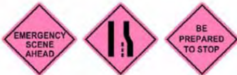
Figure 7 - Example Advance Warning Signs
