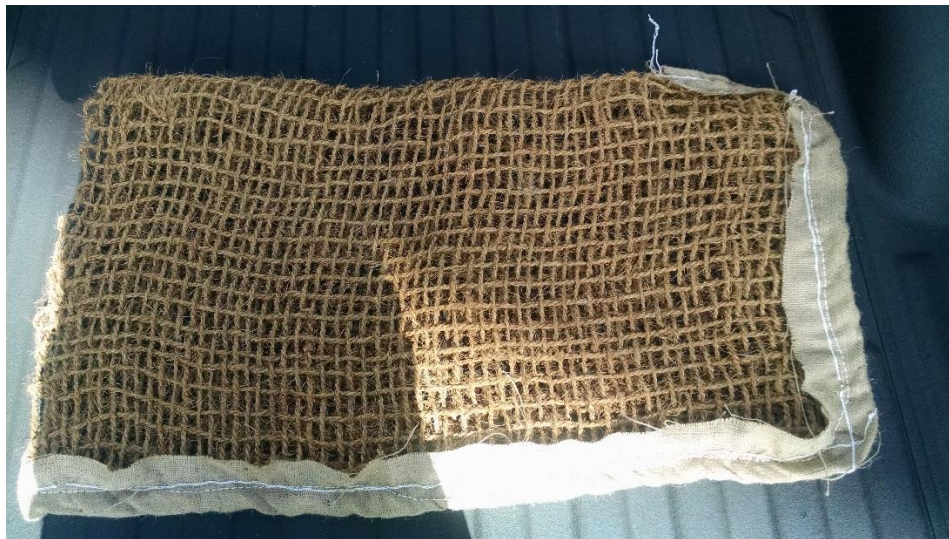
Figure 2: Oyster Shell bag made of biodegradable coir fiber mesh and sealed on the edges with burlap sewed on with a sewing machine.
