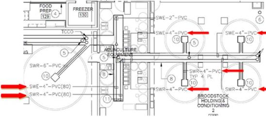
**Response:** The SWE and SWR piping in question in snapshot should be schedule 40 pvc. Also note that SWE piping under driveway, near column 2C should be SWE-6"-PVC(80), not schedule 40.
