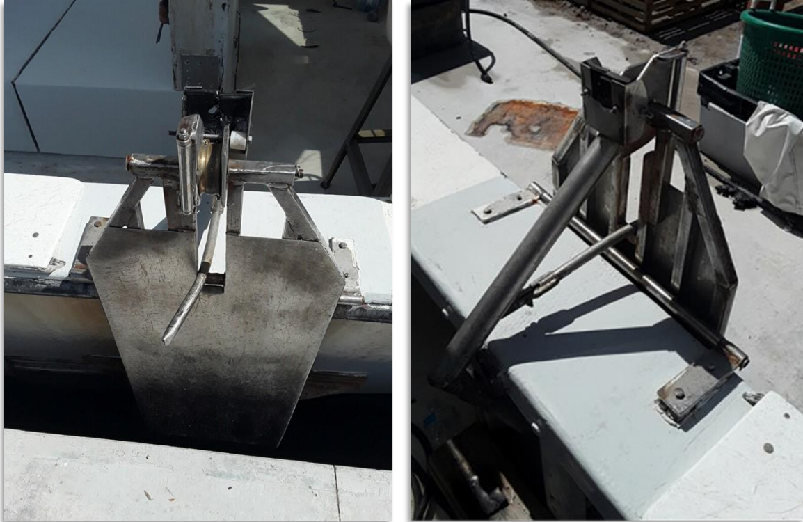
Example of Figure 3. Starboard side gunwale mounted trap tilt table with armature
